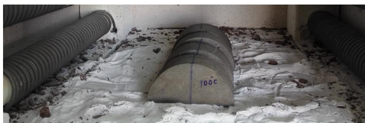
Figure 7. The placement of the specimens in the electric furnace
