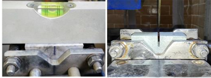
Figure 5. Notching the rock specimens
