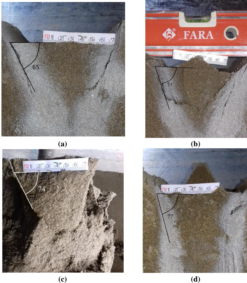
Figure 12. Photos of failure wedges for unreinforced shell foundations with (a) i = 180^\circ , (b) i = 120^\circ , (c) i = 90^\circ and (d) i = 60^\circ
