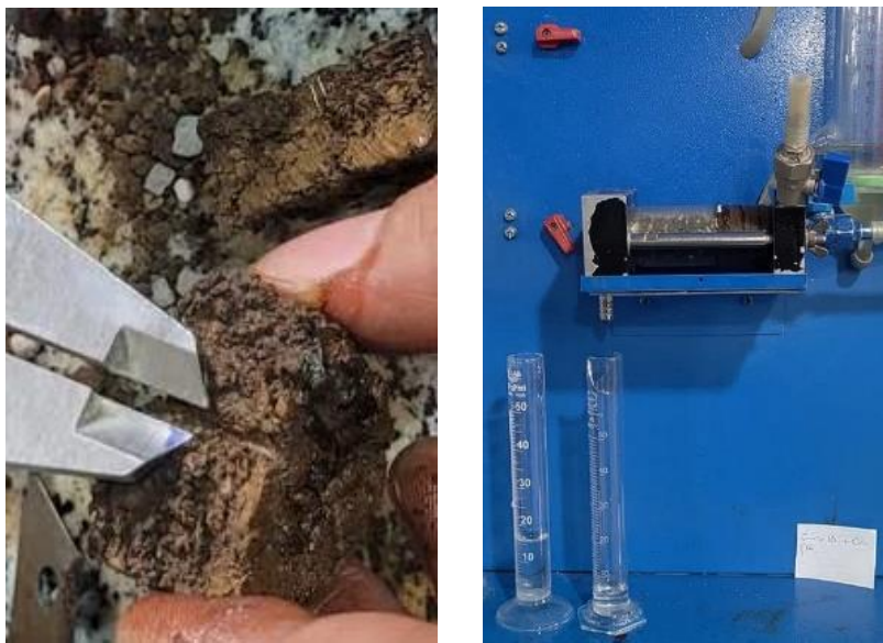
Fig. 2. Images of tests to determine soil dispersivity by pinhole method
