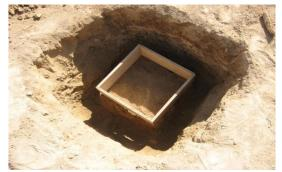
Figure 3. Monolithic sampling method
