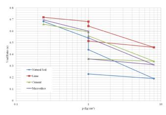
Figure 8. Comparison between natural soil consolidation curve and injected samples
