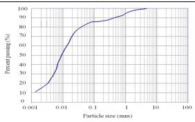
Figure 6. Grain size distribution curve of soil
