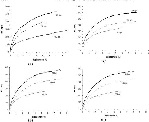
Figure 9. Stress-strain curves for different samples, (a). Natural soil (b). Lime injected soil (c). Cement injected soil (d). Micro silica injected soil
