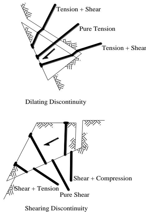
**Figure 5. Reinforcement behavior at discontinuity [2, and 30]**
