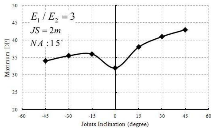
**Figure 21.** Effect of joints dip on maximum DPI
