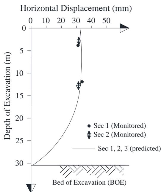
**Figure 8. Comparison between results of FE model and monitoring data**
