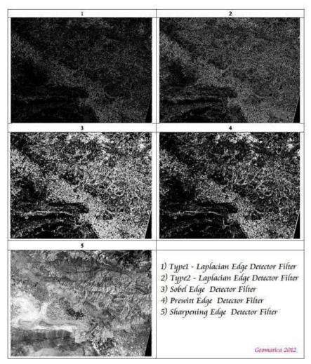
Figure 2. Filtering Method (High Pass)
