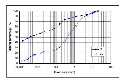
Fig 2: Grain size distribution of the soils
