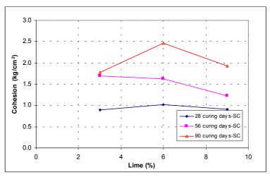
Fig.11: Effect of hydrated lime on cohesion of SC soil
