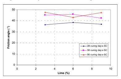
Fig.9: Effect of hydrated lime on friction angle of SC soil
