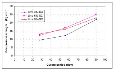
Fig 6: Effect of curing period on compressive strength of SC soil
