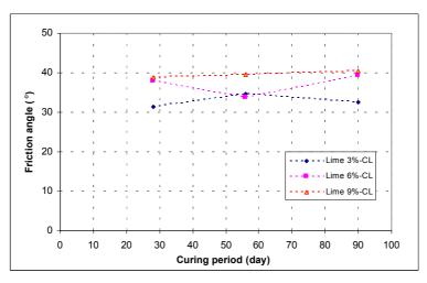
Fig.14: Effect of curing period on friction angle of lime treated CL soil
