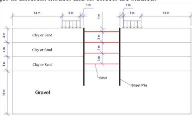
Figure 3. Model geometry
