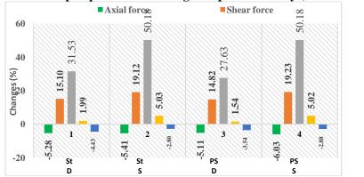
Figure 12. Sheet pile parameters changes in percent - Sand (model No.1)
