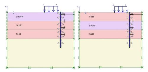
Figure 4. Excavation model with top loose layer (Model 1)
