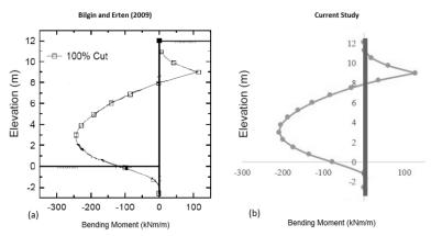
Figure 2. Bending moment acting on sheet pile wall
