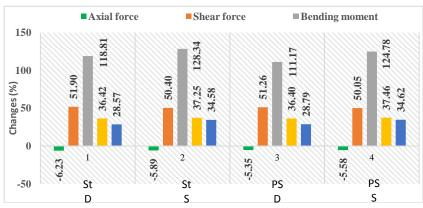
Figure 14. Sheet pile parameters changes in percent - Sand (model No.3)
