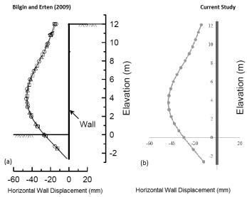
Figure 1. Lateral displacement of sheet pile wall
