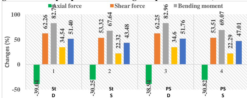
Figure 13. Sheet pile parameters changes in percent - Clay (model No. 3)
