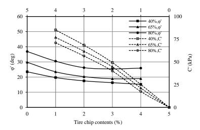
Figure 10. Variation of  $\varphi'$  and C' with tire chip contents and relative density
