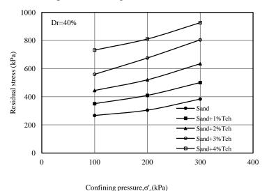
Figure 7.Effect of confining pressure on residual stress for different tire chip contents
