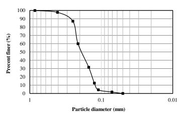
Figure 1. Grain size distribution of sand Tire chips
