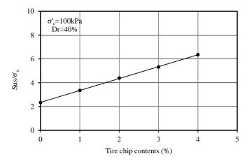
Figure 12. Normalized residual shear strength versus tire chip contents
