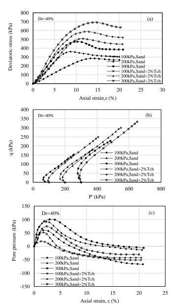
Figure 6. Effect of confining pressure on a) residual stress, b) effective stress path and c) pore water pressure for sand with 2% tire chip contents
