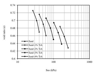
Figure 11. Steady state lines
