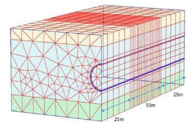
Figure 6. Three-dimensional model of section A
