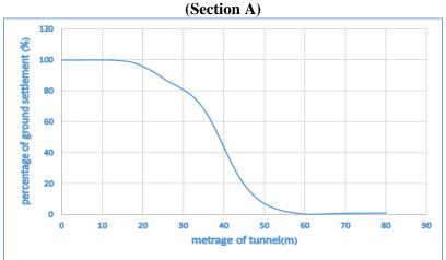
Figure 12. Settlement percentage for a face pressure equal to 1.5 times of the initial face pressure  $(150 \ kPa)$  (Section A)
