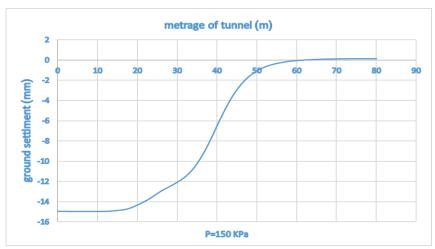
Figure 8. The profile of settlement for a face pressure equal to 1.5 times of the initial face pressure (150 kPa) (Section A)
