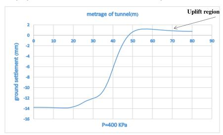
Figure 10. The profile of settlement for a face pressure equal to 4 times of the initial face pressure (400 kPa) (Section A)
