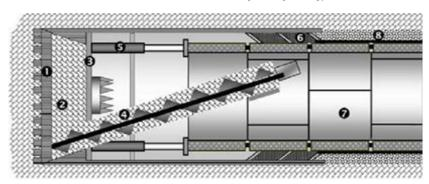
1- Cutterhead; 2- Pressure chamber; 3- Pressure wall; 4- Screw conveyor; 5- Thrust arm; 6- Tail sealant; 7- Segments; 8- Annulus grout Figure 2. Schematic of EPB machine [1]
