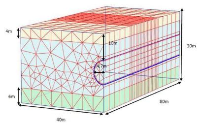
Figure 5. Three-dimensional model of section A built by PLAXIS 3D TUNNEL
