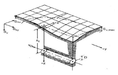
Figure 3. Geometric shape of tunneling-induced ground settlement [4]
