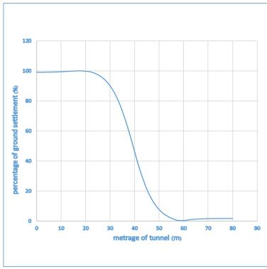
Figure 11. Settlement percentage for the initial face pressure (100 kPa)  $\,$
