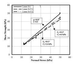
Figure 10. Failure envelopes for  $S_cT_1$  and  $S_cT_2$
