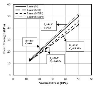
Figure 14. Failure envelopes for  $S_c, S_cT_1, S_cT_1P_c$  and  $S_cT_1P_f$ .
