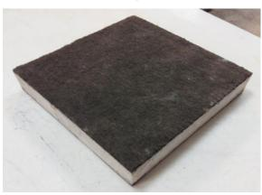
Figure 3. Teflon with attached geotextile
