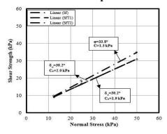
Figure 12. Failure envelopes for  $S_cT_1$  and  $S_cT_2$
