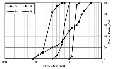
Figure 1. Soil particle size distribution curves
