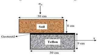
Figure 4. Geotextile position
