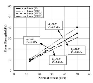
Figure 20. Failure envelopes for S<sub>f</sub>, S<sub>f</sub>T<sub>2</sub>, S<sub>f</sub>T<sub>2</sub>P<sub>c</sub> and S<sub>f</sub>T<sub>2</sub>P<sub>f</sub>.
