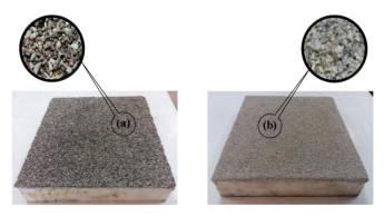
Figure 6. Coarsened geotextile; surface with sands: a)  $P_c$  and b)  $P_{\rm f}$
