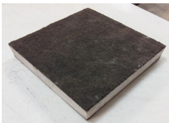
Figure 3. Teflon with attached geotextile
