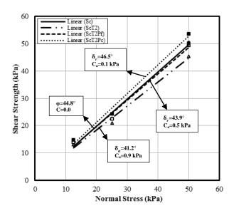
Figure 16. Failure envelopes for  $S_c, S_cT_2, S_cT_2P_c$  and  $S_cT_2P_f$ .
