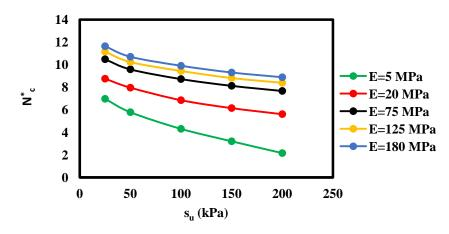
Figure 21. Coupling effect of soil undrained shear strength and elastic modulus on the factor of  $N_{\ c}^{\ast}$
