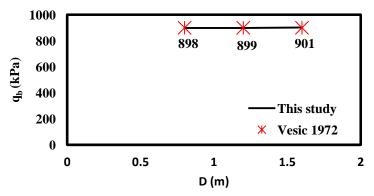
Figure 14. Effect of pile diameter on tip resistance
