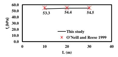
Figure 11. Effect of pile length on side resistance
