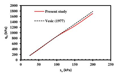
Figure 4. Comparison of tip resistance obtained in this study with relationships suggested by other researchers which are based on soil geotechnical parameters
