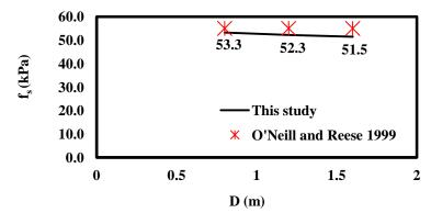
Figure 15. Effect of pile diameter on side resistance
