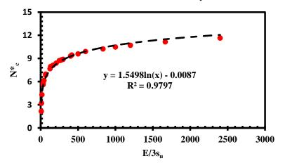
Figure 22. Best curve for values of  $N_c^*$ Table 4. Comparison of  $N_c^*$  proposed in this study with  $N_c^*$  proposed by Vesic (1977)
