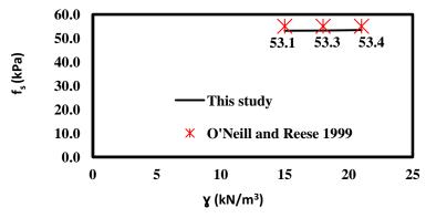
Figure 13. Effect of soil unit weight on side resistance
