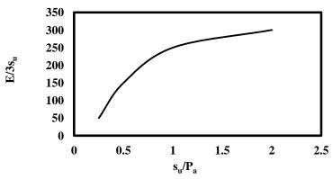
Figure 1. values for soil rigidity index based on undrained shear strength (O'Neil and Reese (1999))
