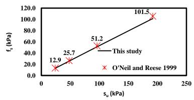
Figure 9. Effect of soil undrained shear strength on side resistance
