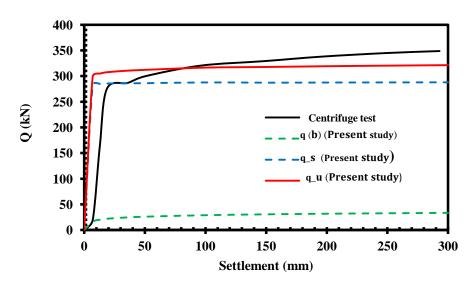
Figure 3. Comparison of the results obtained in this study with the results of the centrifuge test conducted by Horikoshi and Randolph (1996)
