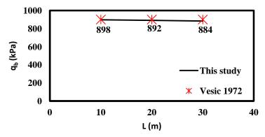
Figure 10. Effect of pile length on tip resistance
