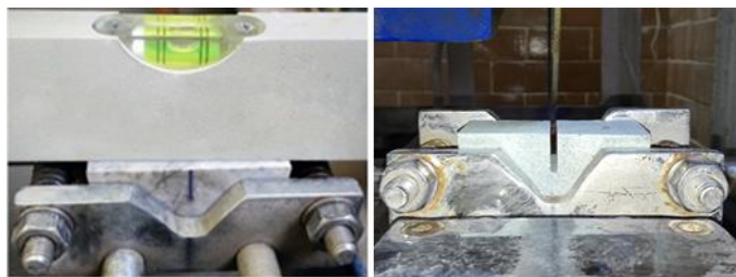
Figure 5. Notching the rock specimens
