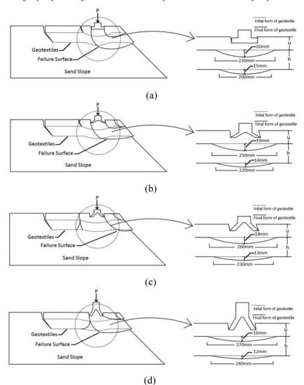
Figure 9. Failure mechanisms of shell foundations with apex angle (a)  $i=180^{\circ}$ , (b)  $i=120^{\circ}$ , (c)  $i=90^{\circ}$  and (d)  $i=60^{\circ}$  on reinforced slope for x/B=1.0 (left side for failure surfaces and right side for exerted deformations in geotextiles)
