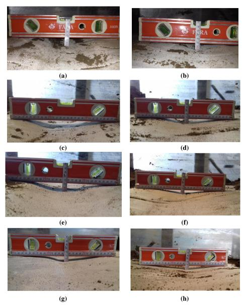
Figure 8. Deformation of geotextile layers beneath shell foundations (edge distance of 2B) on reinforced slope with apex angle (a, b)  $i=180^{\circ}$ , (c, d)  $i=120^{\circ}$ , (e, f)  $i=90^{\circ}$  and (g, h)  $i=60^{\circ}$  (left side for first layer and right side for second layer of the geotextiles)
