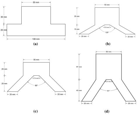
Figure 2. Geometrical configuration of footings
