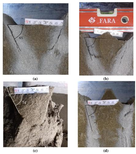
Figure 12. Photos of failure wedges for unreinforced shell foundations with (a) i=  $180^{\circ}$ , (b) i=  $120^{\circ}$ , (c) i=  $90^{\circ}$  and (d) i=  $60^{\circ}$
