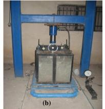
Figure 5. Vibratory tamper and test box during loading (a) Vibratory tamper (b) Loading frame and test box
