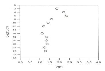
Fig. 6: Relationship between CPI (Carbon preference index) anceepth for samples from the Mostyn Dock site (top) and Mostyn Quay site (bottom)
