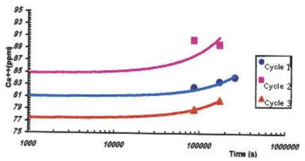
Fig.10. Dissolution of calcium carbonate versus log of time for three phases in carbon dioxide of different concentration. Phase 2 selected for determined of  $K_{\rm c}$ .
