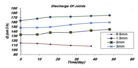
Fig.9. The reduction of water discharge through aperture of 0.5 mm and the increase of water discharge through aperture 1.5, 2 and 3 mm during the testing period.
