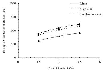
Fig 2. Variation of the isotropic compression yield strength of cemented bonds with cement content.
