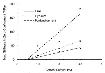
Fig4. Variation of bond stiffness with cement content
