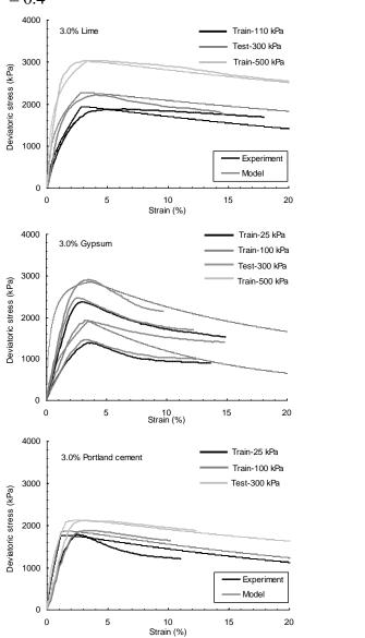
Fig6. Model results for stress-strain behavior of cemented soil in undrained condition
