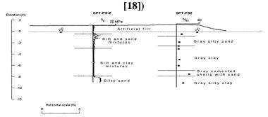
Fig.2. Soil profiling in the Police station site located on the east shore of Izmit Bay, in the town of Golcuk [17]
