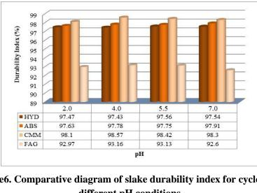
Figure 6. Comparative diagram of slake durability index for cycle 15 in different pH conditions
