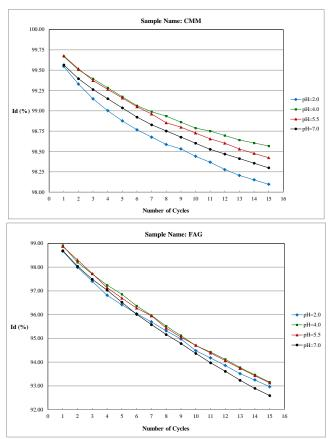
Figure 5. Influence of the number of slaking cycles on slake durability index in different pH conditions
