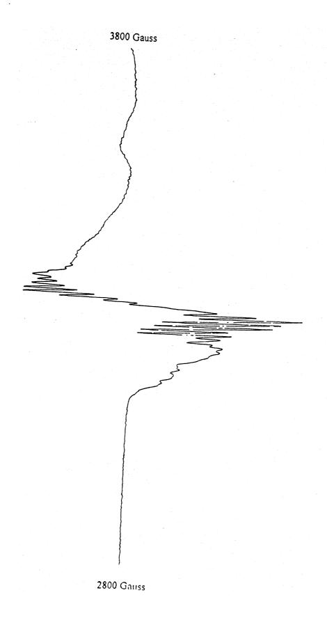
Figure 5: ESR spectra of complex [Cu2L2] at room temperature. The field set was 3300 gauss, and the scan range was 1000 gauss.
