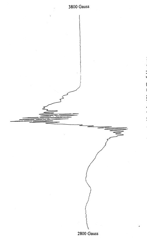
Figure 2: ESR spectra of complex [Cu<sub>2</sub>L<sub>1</sub>] at 130 K. The field set was 3300 gauss, and the scan range was 1000 gauss.
