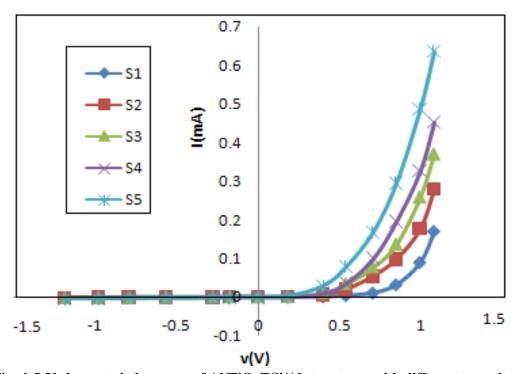
Fig. 4. I-V characteristic curves of Al/TiO<sub>2</sub>/PSi/Al structures with different porosity
