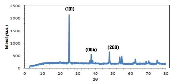
Fig. 2. XRD pattern of TiO2 thin film
