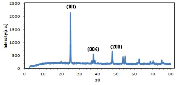
Fig. 2. XRD pattern of TiO2 thin film
