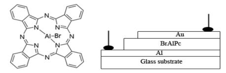
Figure 1. Molecular structure of BrAlPc and schematic diagram of Al-BrAlPc-Au device
