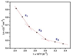
Figure 7. Plot of Ln ( $\sigma$ ) versus 1000/T for Al-BrAlPc-Au device.  $E_1$ ,  $E_2$  and  $E_3$  are activation energies in the intrinsic region and impurity scattering regions, respectively
