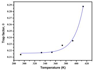
Figure 6. Variation of trap factor  $(\theta)$  with temperature for Al-BrAlPc-Au device. At low temperature, trap factor is relatively unchanged but when temperature increases trap factor changes nonlinearly
