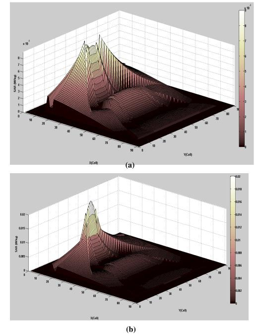
Figure 4. Specific Absorption Rate (SAR) 3 dimensional pattern in x- y plane passing through the source position for, (a) 5 layered model, (b) 6 layered model.
