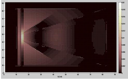
Figure 2. Specific Absorption Rate (SAR) distribution in x- y plane passing through the source position for, (a) 5 layered model, (b) 6 layered model
