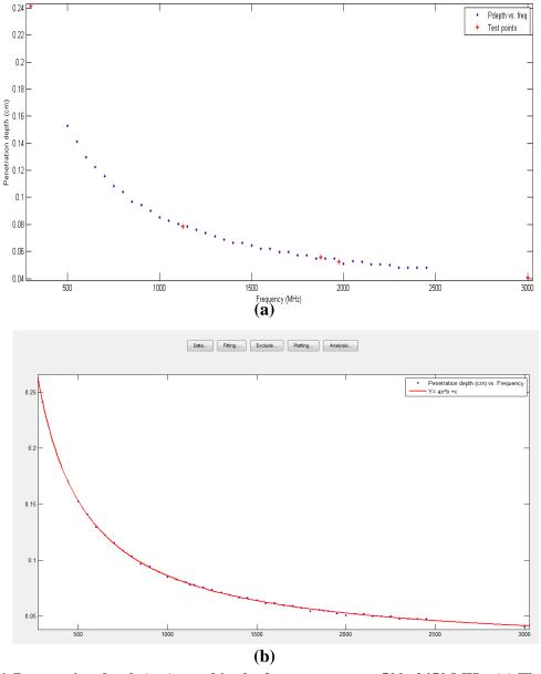
Figure 6. Penetration depth (cm) trend in the frequency range 500- 2450 MHz. (a) The dots are the data gathered in stage 5 from grey matter as a lossy dielectric material, the solid line is achieved by curve fitting, (b) the asterisks are extra data to examine the accuracy of the fitted curve
